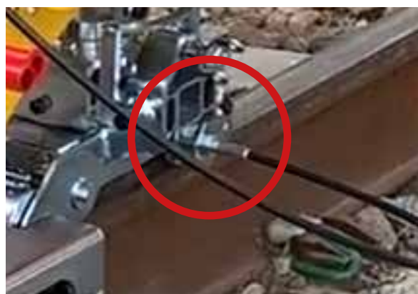
Fig 34. Disconnect the brake wire
