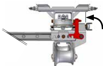
Fig 41. Lock the slide carriage
