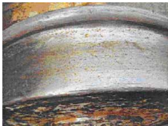
Fig 115. Circumferential cracking limit associated with rollover
