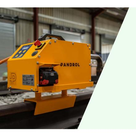
The HFP 36V is battery powered and fully automated for easier, more reliable operation: the ignition, timing and stop require no manual interference or flame adjustment. It uses only propane, no oxygen is required, reducing costs and reducing the total weight to carry on site.
