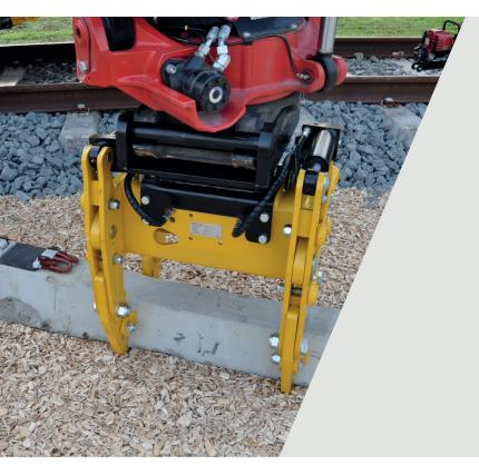
Rosenqvist Rail's Sleeper Grabber SG60 is a highperformance tool for heavy-lifting track procedures.
