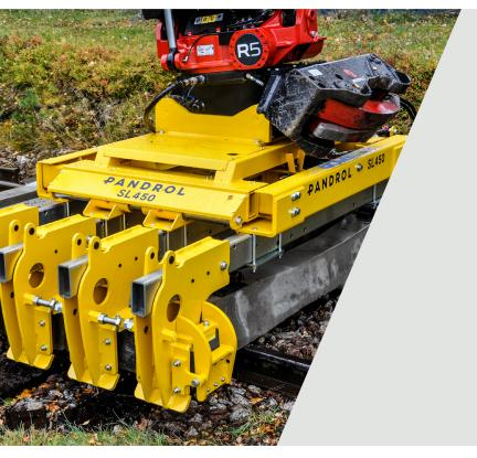
Rosenqvist Rail's range of carrier-mounted Sleeper Layers achieve fast, accurate sleeper laying and spreading, with an easily adjustable tool designed to fit most kinds of sleepers. The SL400 can handle four sleepers simultaneously, while the SL850 can handle up to eight at a time.
