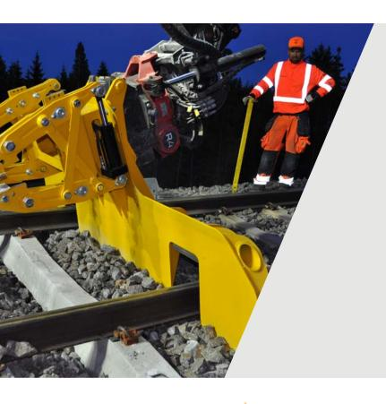
Pandrol's SB40 and SB60 Sleeper Replacers are attachments designed to replace sleepers safely and efficiently.
