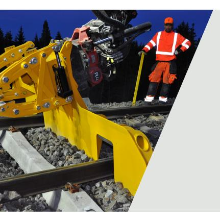
SB40 and SB60 Sleeper Replacers are attachments designed to replace sleepers safely and efficiently.
