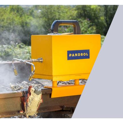
Pandrol's i+cool device is designed to increase welding productivity by cooling welds faster.
