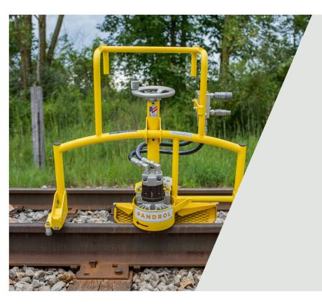
Pandrol's Profile Grinder (06000B) is a lightweight, precision grinding machine.
