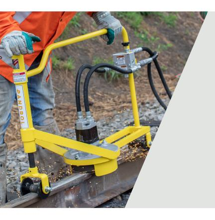
The Surfacing Guide Grinder is a coarse but lightweight grinding attachment designed especially for grinding the top of the rail. It is perfect for the finish grinding of field welds or rail end repairs. For maximum safety, the extended guard offers excellent operator protection
