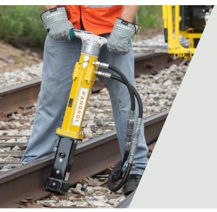
Portable but powerful, the Lightweight Two-Stage Spike Puller weighs only 39lbs but generates an impressive pulling force of 13,000lbs.
