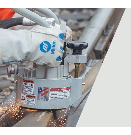
The Pandrol 6" Cup Stone Grinder is a versatile tool designed for grinding the tops of frogs and the rail.
