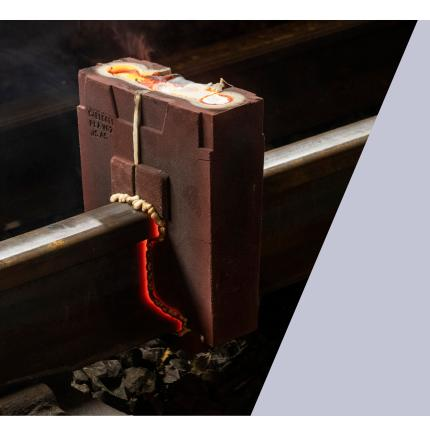
Pandrol's i+seal – the world's first self-sealing mould – significantly streamlines the aluminothermic welding process.
