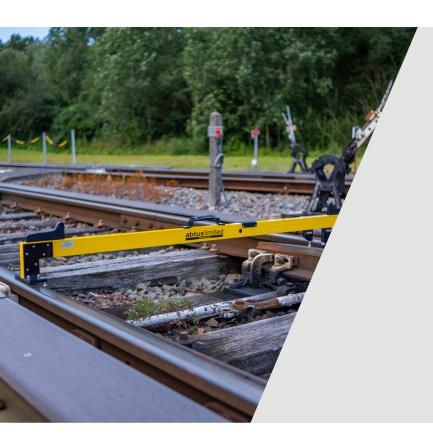
The P8 Inspector's Gauge (P5020) is a lightweight, multipurpose track gauge that delivers accurate and repeatable measurements on plain line and in areas of switch and crossing.
