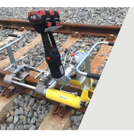
Pandrol's battery-operated weld shearing machines are designed for the easy removal of excess metal following an aluminothermic weld. The shearing process takes place after mould release.
