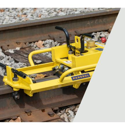
The Pandrol Weld Shear is designed to make it easier and more efficient to remove excess weld metal.
