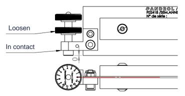
• Turn the setting wheel in clockwise direction to give the value of the level point desired. For example, 0.66mm
