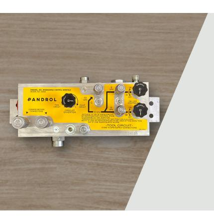
The Hydraulic Manifold Circuit is a self-contained flow and directional control assembly. Compact and easy to install, this manifold provides a safe and cost-effective way of adding hydraulic tool capabilities to your existing range of equipment. Suitable for any vehicle equipped with a hydraulic system capable of producing at least 10 gpm at 2,000 psi.
