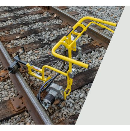
Pandrol's Multi-Purpose Grinder (06950) is a versatile tool that is suitable from field grinding to switch points and frogs.
