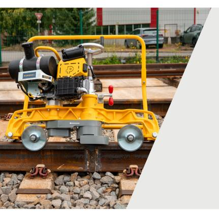
The Pandrol SolidGrinder-P-150-VIR has been designed to fully grind the rail head after welding. Like all of Pandrol's grinding machines, it combines power and reliability with ease of use.
